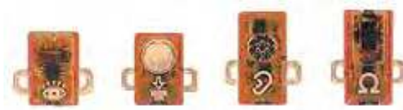
Cricket Sensors: Light sensor, touch sensor, sound sensor, resistance sensor.
